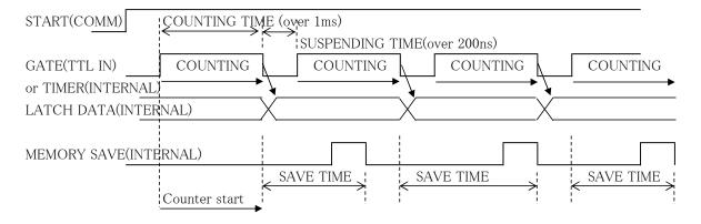
To meet the condition of SAVE TIME >= 1ms, with ECC time(4ms) , please input COUNTING TIME + SUSPENDING TIME >= 5ms.
