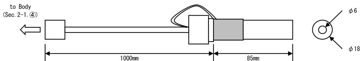
The sensor is attached to the gauge port of φ18.
